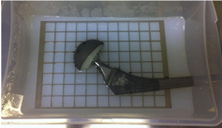
Figure 11: Image showing the prosthetic half-submerged in agarose gel along with the plexiglass grid. Taken from [14] with permission from the publisher (Elsevier). For scale, the box is approximately 20cm by 30cm.
