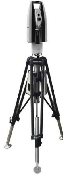
Figure 3. Leica Absolute Tracker
