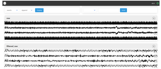
Figure 10. Monitor showing real time data: the top plot represents the raw initial data, and the bottom one after being filtered with a band-pass filter
