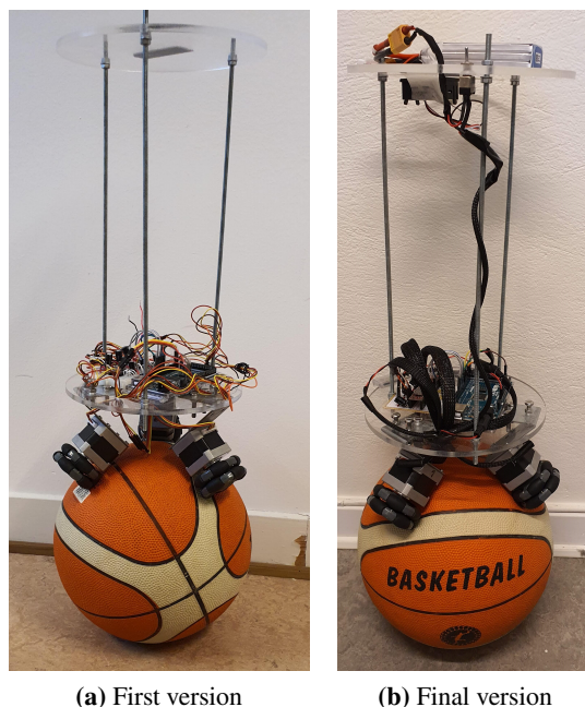
Figure 1. First and final versions of the self-balancing robot.
