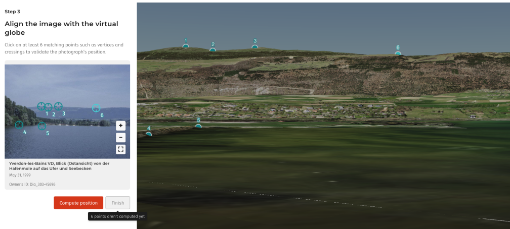
Figure 3.11: The virtual globe is then shown and the user is asked to identify the GCPs, in the historic photo (to the left) and in the virtual globe (to the right) [4]
