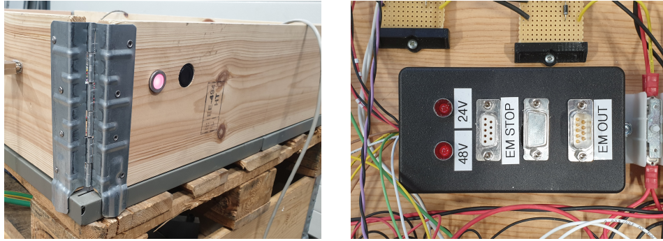
(a) Light to indicate the status of the RT7 safety relay, where red means stopped and green means active, with the reset button to the right.
