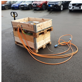
(b) Test pallet outside due to smoke emerging from the lower pallet.
