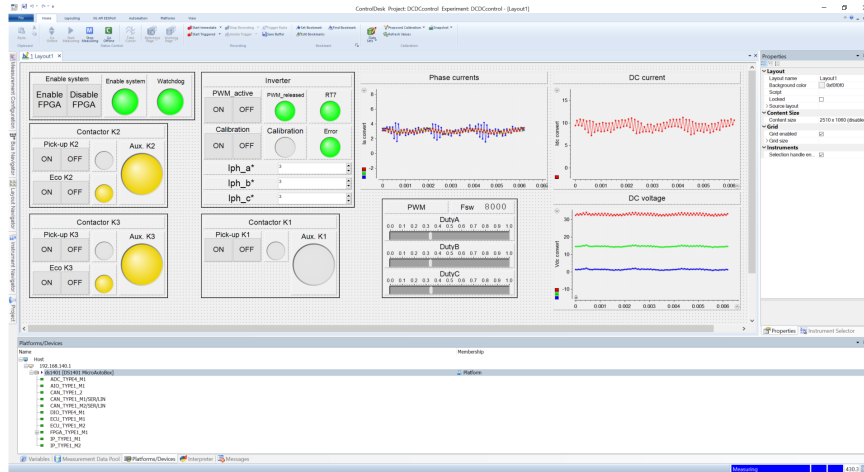
Fig. 3.10. The dSpace Control Desk layout used for testing each current controller separately in boost mode with a resistive load. Note that the DC current measures the sum of the phases instead of the load current. This is resolved in all further testing.
