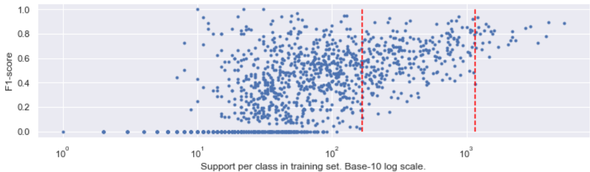
Figure 5.9: F 1 -score per class based on class support for XLM-R model on oversampled data with a sampling threshold of 50.
