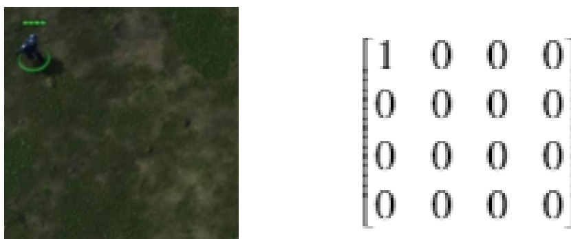
Figure 2.3: A approximately 21x21 game window and a simplification of the corresponding player_relative matrix, in reality the matrix would be in a higher resolution.
