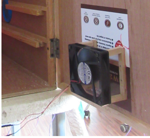
Figure 3.3a: A stand used to attach a fan when using the bottom inlet (green circle in figure 3.1). The space between the fan and the wall is of 5 cm to 5.5 cm.
