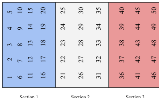
Figure 7.2b: Diagram showing the labelling of the samples for a tray with 50 samples.
