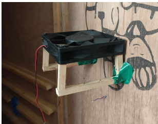
Figure 3.3b: A stand used to attach a fan when using the top inlet (red circle in figure 3.1).
