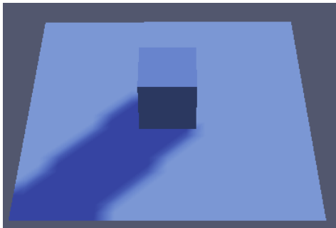
qr field in case without cyclic boundaries, calculated using the standard solarLoad library
