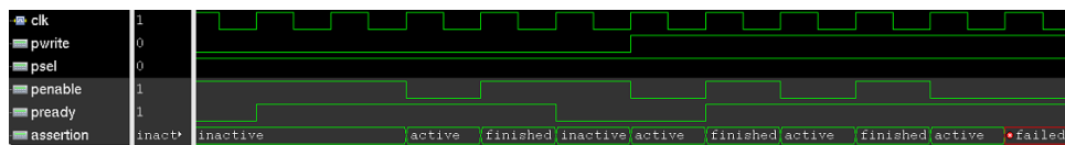
Figure 3.17: A simple waveform of APB with assertions.
