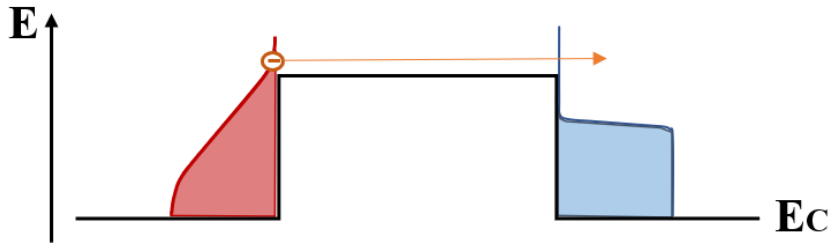
Figure 8: An illustration of a rectangular barrier with a temperature difference across the barrier, with the Fermi distribution functions indicated on either side of the barrier.
