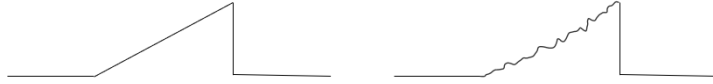
Figure 44: An illustration of the band structure with an ideal, smooth, ratchet-like barrier (left) and a more realistic, rugged, barrier (right).
