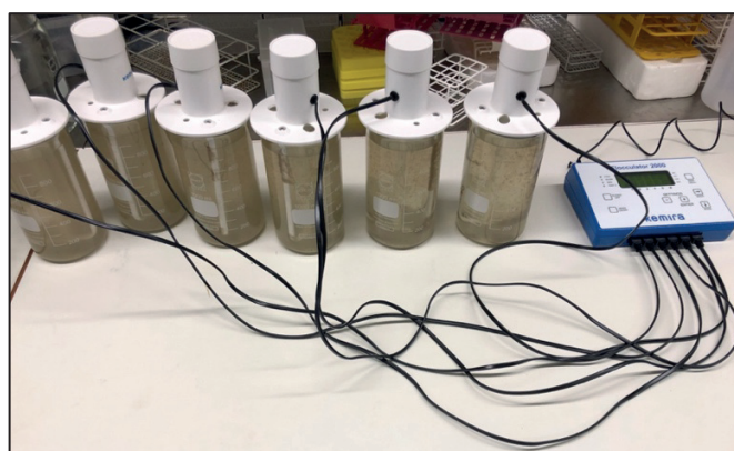
Figure 3.2 Jar-Test set-up. Each jar has a mixer that is connected to a control device.
