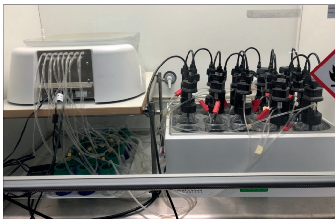
Figure 3.2 The AMPTS set up. To the left, the Gas Volume Measuring device above the CO 2 -fixating devices. To the right, the reactors with motors and stirrers are placed inside the heated water bath. The entire set-up is contained inside a fume hood.
