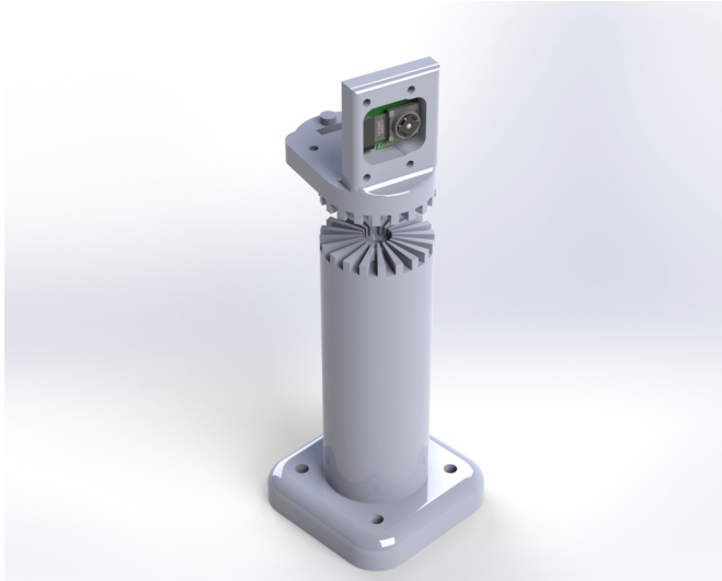
Figure 3.12: Camera mount consisting of two parts to be able to adjust direction in increments of 16^\circ .
