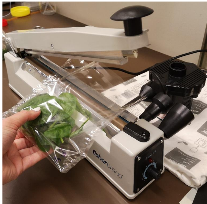
Figure 3. Process of sealing packages while pumping air in the bag with an electrical air pump.
