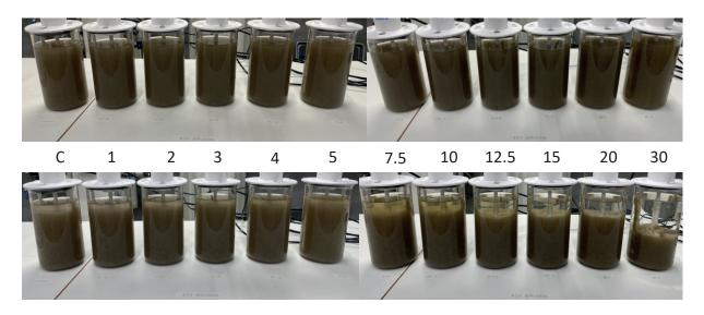
Figure 6.6 Jar Test for biologically treated greywater using PIX-111 during slow mixing (upper) and after settling for 30 minutes (lower). Molar ratios listed in between the two timepoints.
