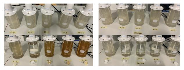
Figure 5.3 Jar tests on influent greywater using PIX-111(left) and PAX-XL60 (right) during the proof of concept stage.
