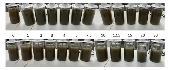
Figure 6.7 Jar Test for biologically treated greywater using PAX-XL60 during slow mixing (upper) and after settling for 30 minutes (lower). Molar ratios listed in between the two timepoints.
