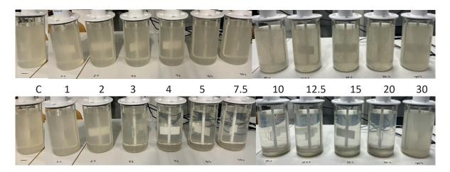
*Figure 6.2 Jar Test for influent greywater using PAX-XL60 during slow mixing (upper) and after settling for 30 minutes (lower). Molar ratios listed in between the two timepoints.*
