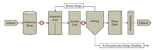
Figure 3.1 Treatment scheme for greywater at RecoLab pilot plant for Oceanhamnen during the spring of 2022. Sampling points circled in red.
