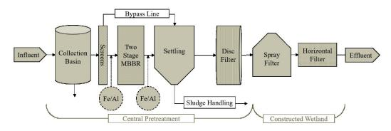
Figure 3.2 Treatment scheme at the proposed Östra Ramlösa plant. Proposed chemical precipitation points denoted with dotted lines (simplified, coagulation and flocculation tank placement decided upon final precipitation placement decision).
