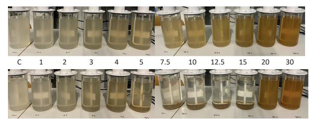
Figure 6.1 Jar Test for influent greywater using PIX-111 during slow mixing (upper) and after settling for 30 minutes (lower). Molar ratios listed in between the two timepoints.
