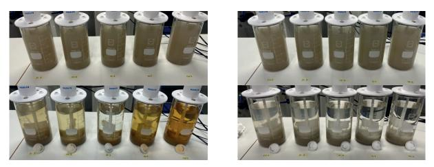
*Figure 5.4 Jar tests on biologically treated water using PIX-111(left) and PAX-XL60 (right) during the proof of concept stage.*
