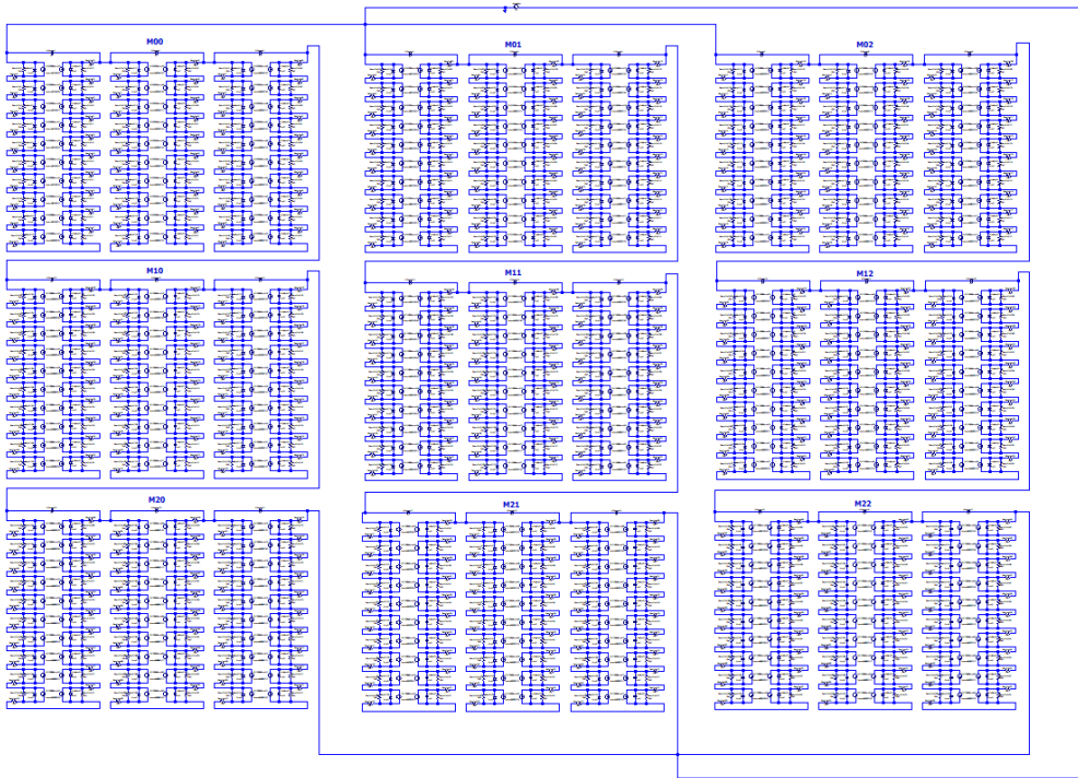
Figure 3.3: LTspice model of a PV array. (8)
