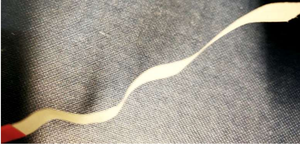
Figure 5.2: Wrinkles in TFA sample after testing
