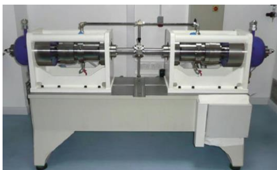
Figure 4. Twin-piston rapid compression machine located in the Combustion Chemistry Centre of NUI Galway. Source of the figure: p. 168. of the book of Battin-Leclerc et al. [51]
