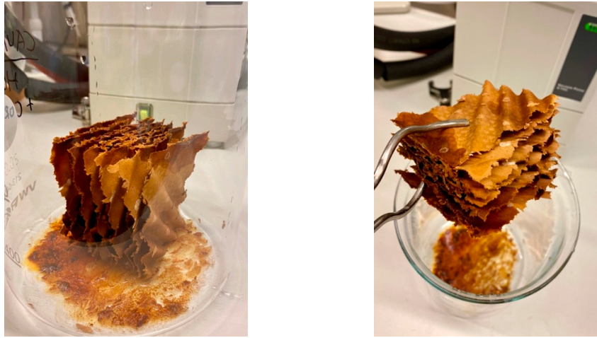
Figure 15: Result of 25 days packing material test in sodium hydroxide solution.
