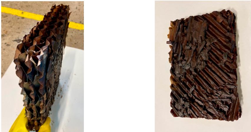
Figure 16: Evaporative block after serial runs on black liquor at high temperatures and concentrations.
