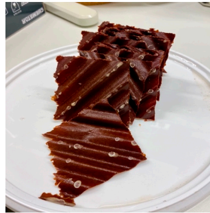
Figure 14: Cellulose test result after 48 hours. Resin dissolution between corrugated paper sheets.
