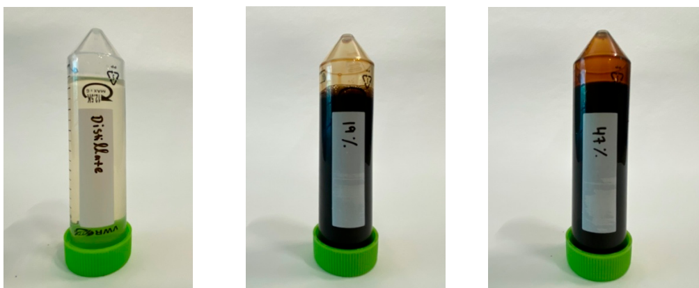
Figure 24: Distillate from pilot unit and black liquor at 19% and 47% dry substance from experimental runs.
