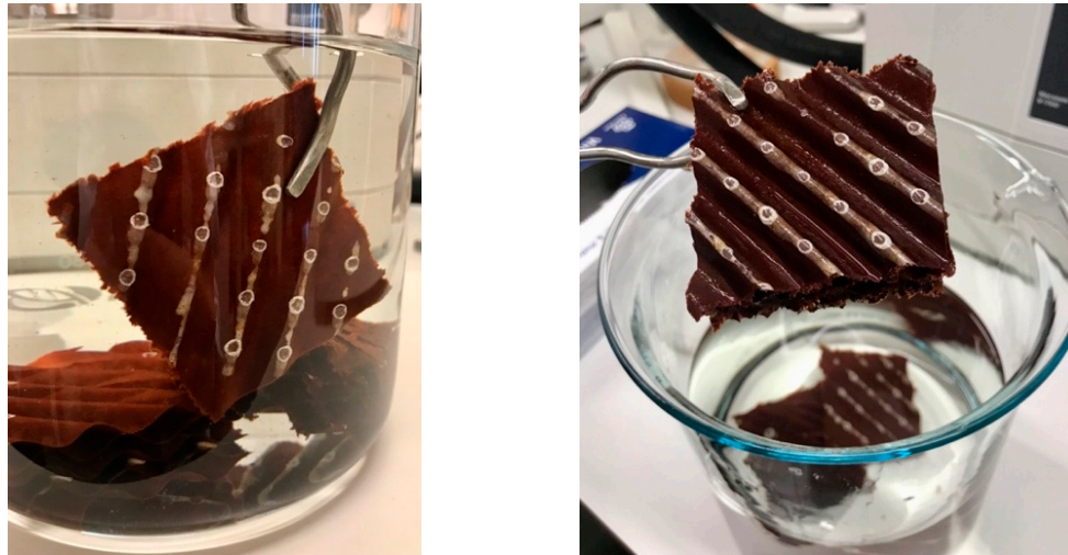
Figure 12: Cellulose test result after 24 hours. Resin dissolution between corrugated paper sheets.
