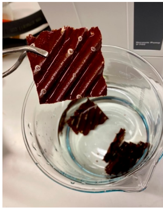
Figure 14: Cellulose test result after 48 hours. Resin dissolution between corrugated paper sheets.
