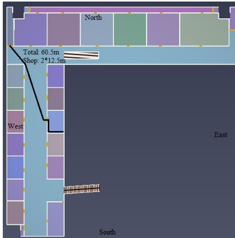
Figure 3. First floor of the simulation model. Black lines represent the longest escape routes.
