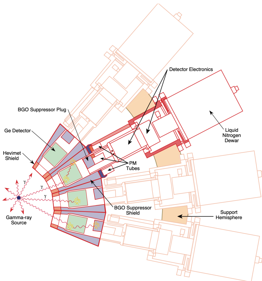
Figure 3.4: A schematic drawing showing the side-view design of GAMMASPHERE [19].
