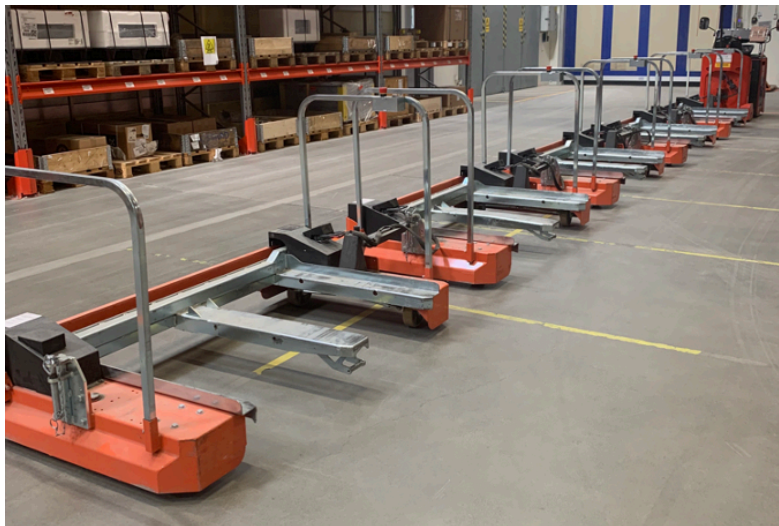
Figure 28. “The train” that distributes load carriers.
