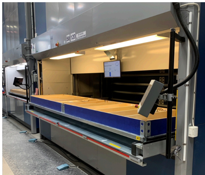
Figure 22. Vertical storage lift 50 with a retrieved shelf.
