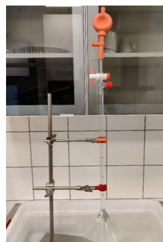
Figure 6. Water bath, burette and pileus ball used for headspace volume measurements
