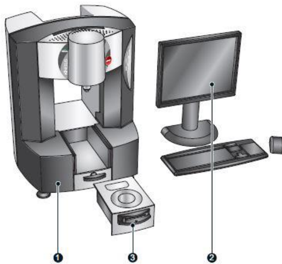
Figure 11: Rheometer Unit: 1. The Rheometer Device, 2. The Controlling Computer 3: Environmental Controller Cartridge [52].
