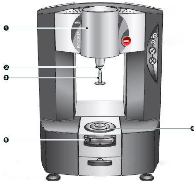
Figure 12: Rheometer device: 1. Head, 2. Chuck, 3. Upper geometry, 4. Lower geometry, 5. Cartridge [52].
