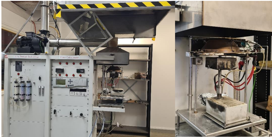
Figure 17: Set-up of the cone-calorimeter apparatus
