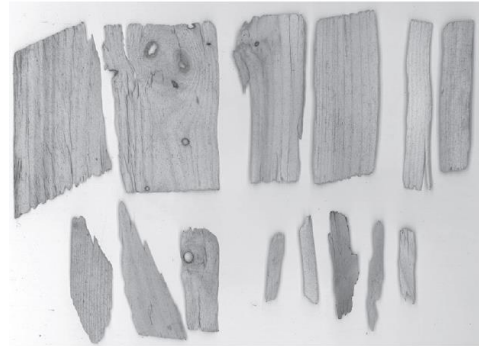
Figure 7: Strand types in OSB Reproduced from [20] with the permission from Elsevier
