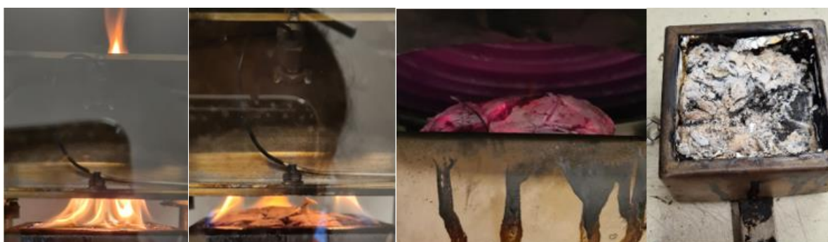
Figure 26: OSB3 sample during cone calorimeter test and afterwards
