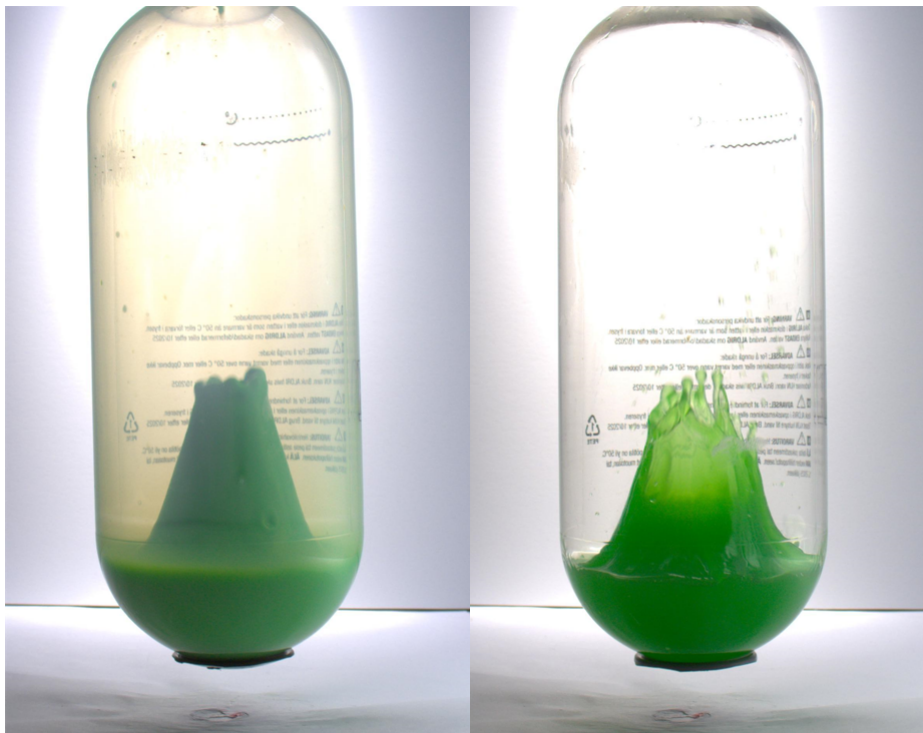
Figure 28: Milk (left) and water (right) in corresponding frames for drop height 8 cm with fill level 4.5 cm.
