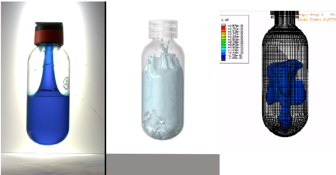
Figure 1: Illustration of a physical drop test (left), a current virtual twin (middle), and a virtual twin from 2013 (right).
