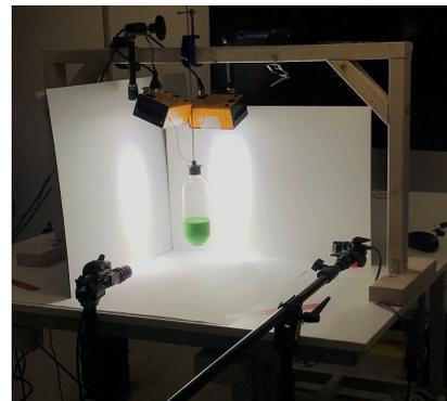
Using image analysis and computer vision algorithms we could produce 3D reconstructions of the surface of the liquids during these drops. This data was then fed to a type of neural network called a U-Net, which after training could predict the motion of the liquid, being told only which height the bottle was dropped, the fill level, and type of liquid. In the figure a drop image, the 3D reconstruction, and the prediction a drop image from the U-Net is illustrated for never-seen-before data.
