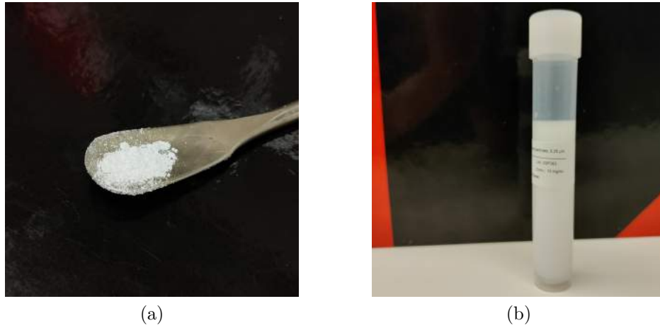
Figure 15: (a) amorphous PLA powder and (b) PLA NPs.
