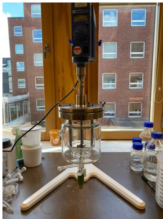
Fig. 6. Setup including torque stirrer attached to the lid with mixer and glass chamber used for acid hydrolysis of the native waxy starches.
