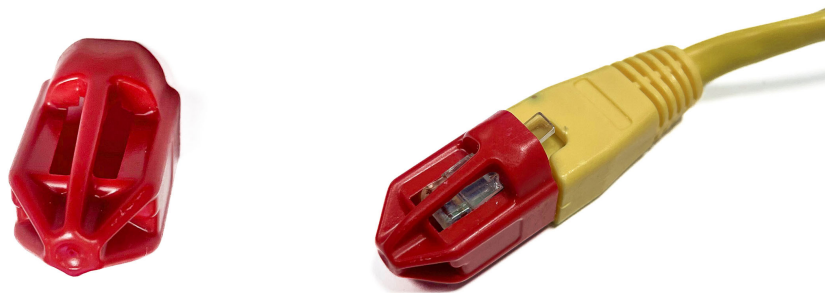
Figure 4.1: The figure shows a picture of the Hannibal tool which is mounted onto a modular plug when pulling the plug through the existing grommets (Cable Gasket 1 and Cable Gasket 2).
