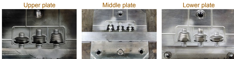
Figure 6.21: The figure shows the family mold used to fabricate prototypes in SiR for concept c4, c13 and c20. The pictures were provided by the supplier.
