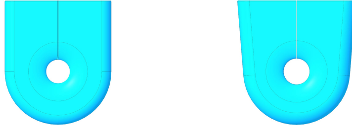
Figure 6.13: The figure shows a 3D model of concept c1. To the left is the first version with straight lines and to the right is the updated version with tilted sides.
