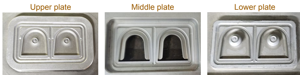
Figure 6.22: The figure shows the mold used to fabricate prototypes in SiR for concept c1. The pictures were provided by the supplier.
