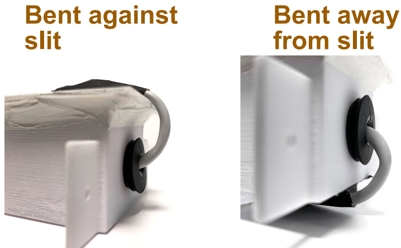
Figure 8.7: The figure shows a test box and how the cable was bent in Test 3 and 4. The slit in the grommet was always positioned up.
