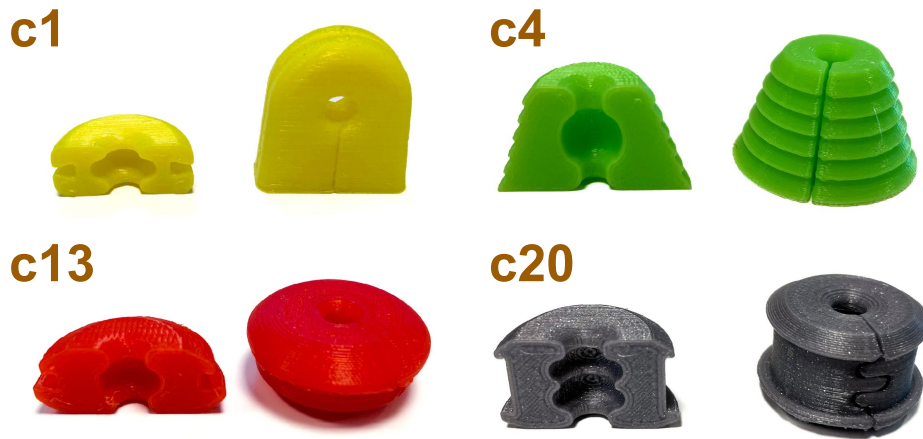
Figure 6.14: The figure shows 3D printed prototypes of concept c1, c4, c13 and c20. The parts were printed in PLA using FFF.
