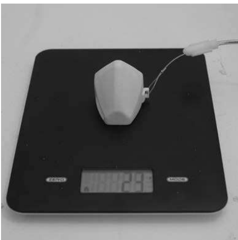
Fixaspine main body with components = 23g
