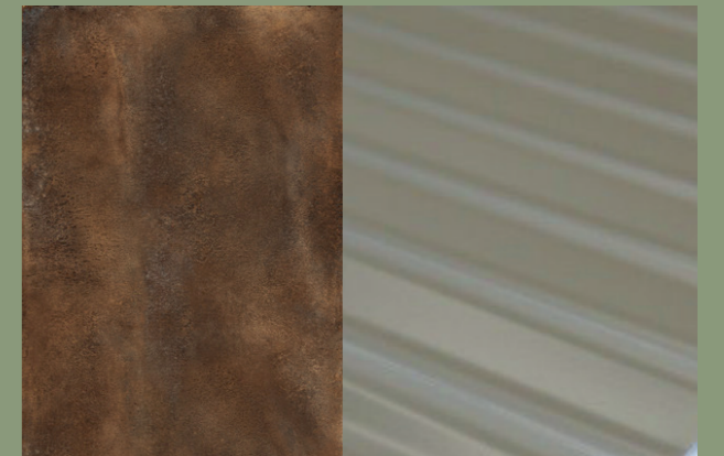
Fig. 35: CorTen steel and corrugated steel sheets
