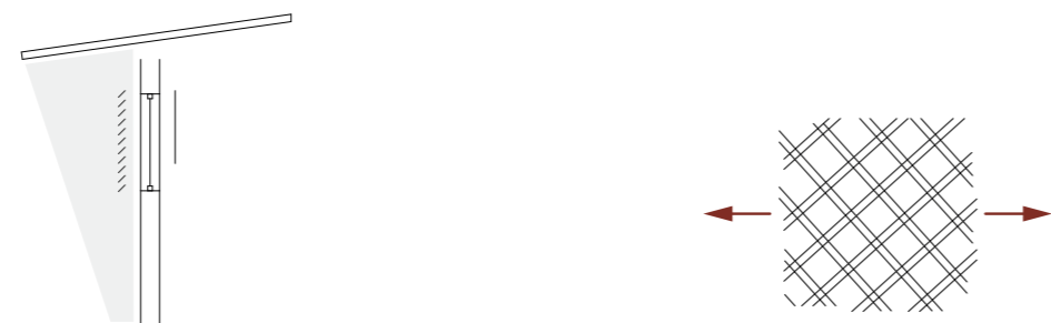
Fig. 45: Example of shading devices on a wall and over openings and perforated movable wall element
