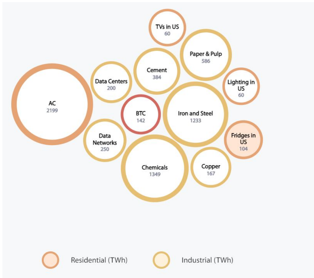
Figure 2.1: Bitcoin energy consumption (BTC) compared to other industrial processes as of March 2022. Comparisons are made on a global scale, if not indicated otherwise, in terms of annual energy consumption (Cambridge Center for Alternative Finance, 2022b).
