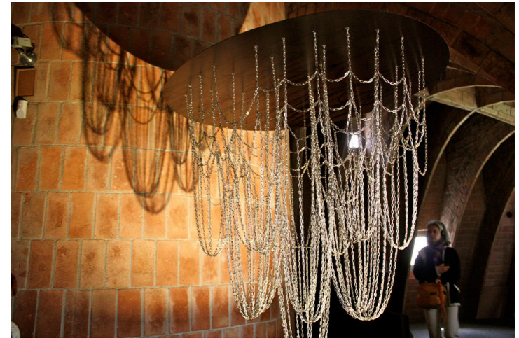
Antoni Gaudi used analog form-finding in his hanging chain models for his vault and dome structures. Digital form finding is likewise about extracting a shape rather than drawing it yourself. (Taylor 2009)
