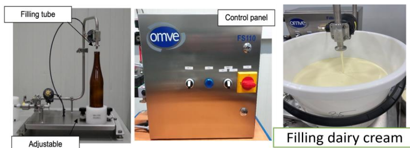
Figure 12 Clean fill system photo from: Omve
