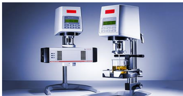
Figure 16 Rotational Rheometer Rheolab, with accessory temperature device, from: Anton Paar, 2022
