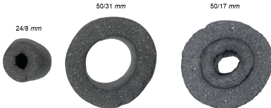
Figure 12.10 Pipe insulations used while testing foams behaviour in profiles.
