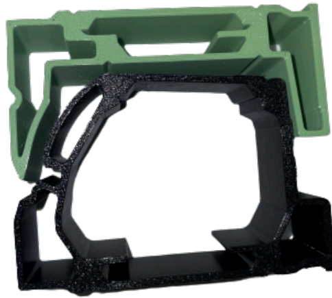
Figure 12.9 Simplified 3D-models of upper and lower stile made in PETG.
