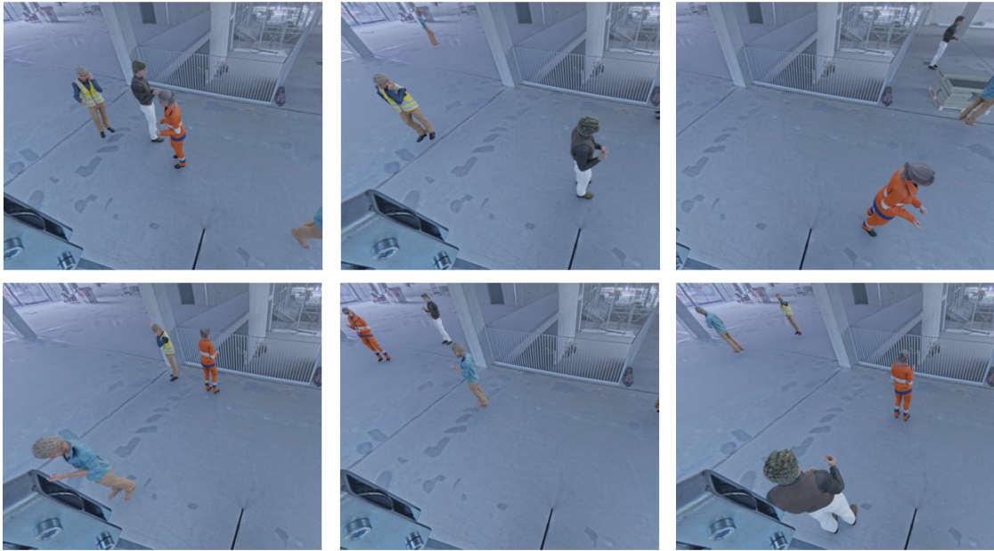
Figure 3.10: Example of the same characters randomly placed within the acceptable ROI of the certain background. The selected characters is placed in the image with a pose. New images in the same iteration are generated by giving the characters new positions and a new pose, before a new iteration with another selection of characters, background, and camera angle is randomized.
