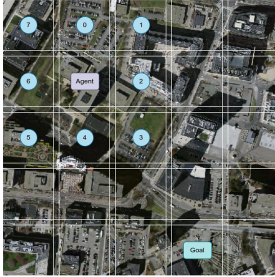
Figure 2: The eight possible actions for the discrete 8-dimensional movement setup (number 0-7 around the agent’s current location). A possible goal location is also indicated.
