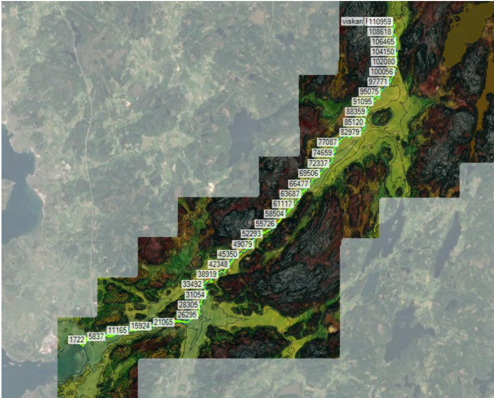
Figure 29. Viskan with assigned cross sections in HEC-RAS Mapper
