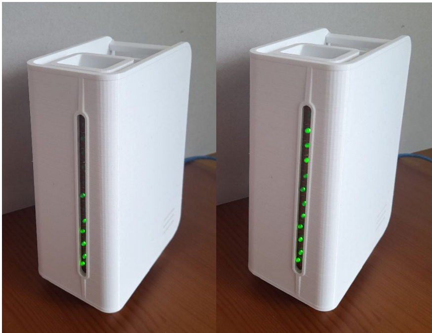
Figure 4.8 & 4.9 The prototype with the LED-strip lit, illustrating time passed.
