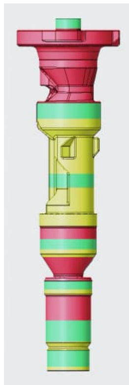
Figure 32, Colouration of how suitable areas are for segmentation. The green areas are the preferred ones, the yellow are not preferred and the red are not suitable for segmentation lines.
