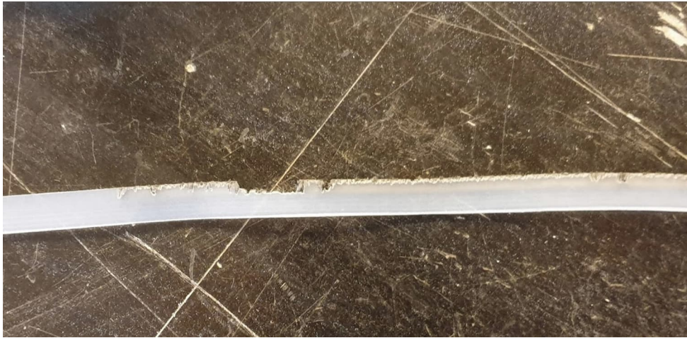
Figure 9, A damaged recoater blade.
