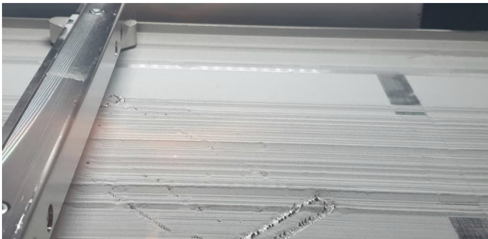
Figure 10, Uneven powder bed as a result of a damaged recoater blade.
