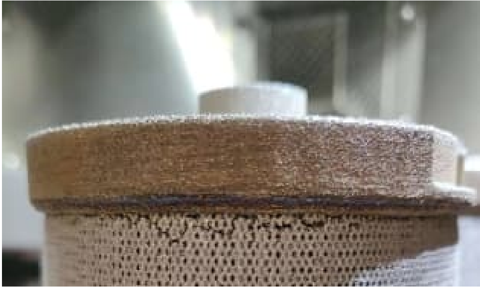
Figure 30, Image of over-melted area and cracking of support structure, courtesy of Alfa Laval.
