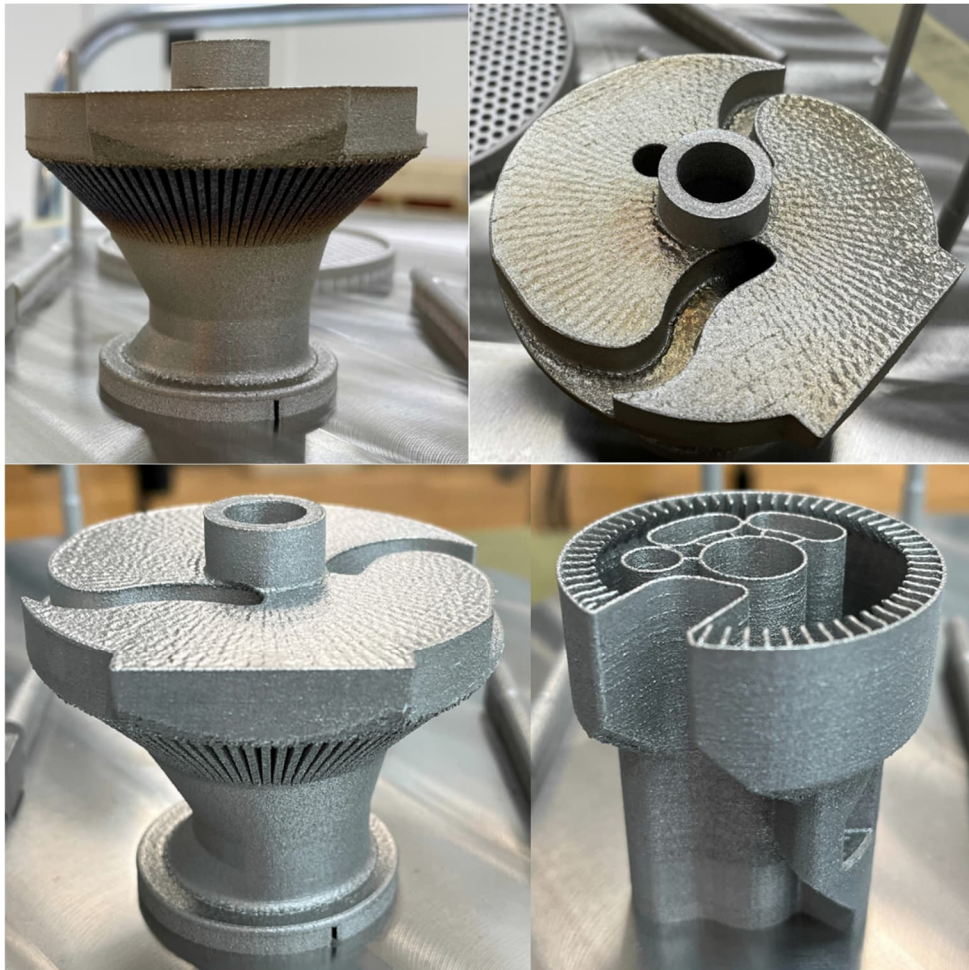
Figure 52, Segment 1 before heat-treatment to the top, and segments 1 and 2 after heat treatment on the bottom.
