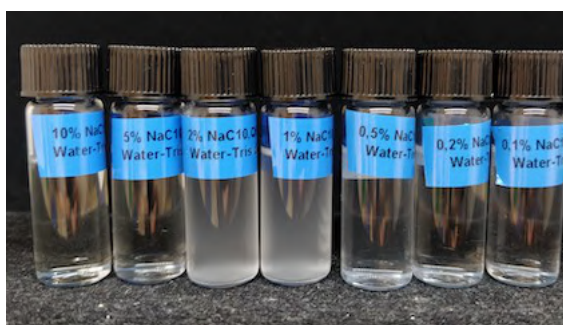
Figure 4.26: Visual appearance for 10, 5, 2, 1, 0.5, 0.2 and 0.1 wt% NaC10-0.1 wt%- Q680 2 wt% with Tris water dilution series.
