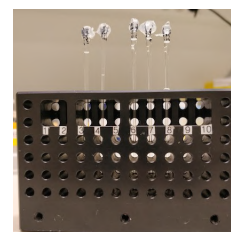
Figure 3.5: Samples filled in glass capillaries that has been sealed with glue on top. The samples are in capillary positions 3, 4 and 6-8 in the sample-holder.
