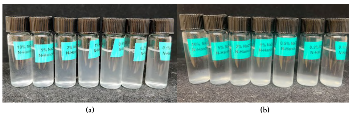
Figure 4.33: Visual appearance of NaClO 10-0.1 wt%- N-Hance 0.5 wt%, series with Tris. (a) Just after preparation. (b) After resting for three days.
