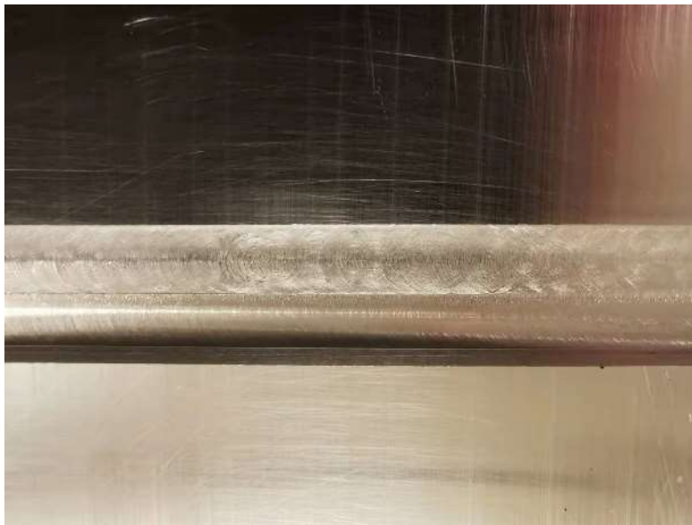
Figure 17: Square feature with vf = 2 \text{ mm/s}
