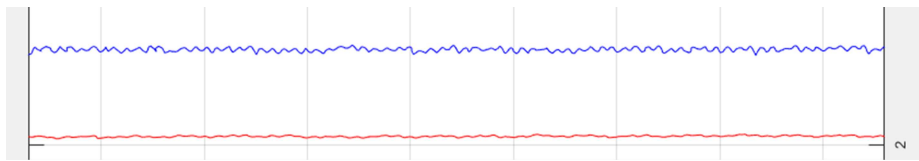
Figure 51: Local path of Line 4 (MRR=1.44cc/min) (Red-air motion; blue-real cut)
