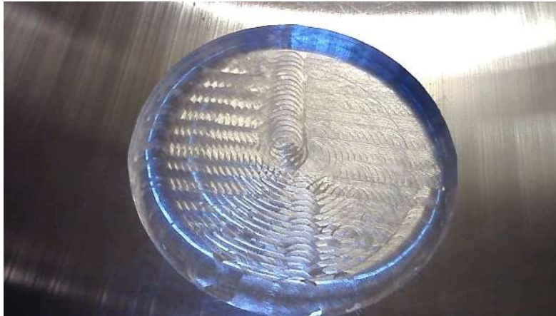
Figure 15: Circle feature with v_f = 2 mm/s
