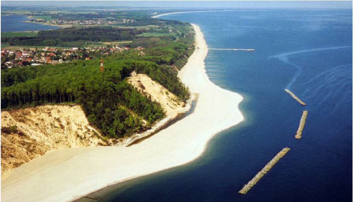
Offshore structures that reduce the power of waves. Image credit: Fröhle & Kohlhasse, 2022
