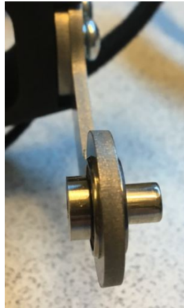
Figure 14: Picture that shows the ball bearing on the orthosis.
