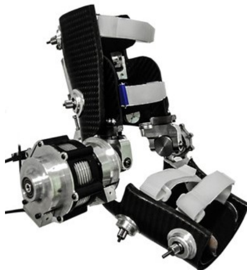
Figure 5: The figure presents an example of a gear driven orthosis [22].
