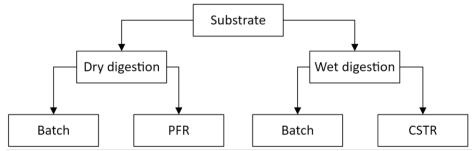
Figure 3. Summary of the reactor types for biogas production
