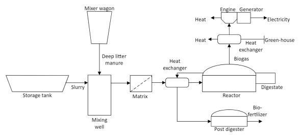
Figure 10. Process from a study visit to cattle farm, Långhult biogas that produce biogas from all types of cattle manure
