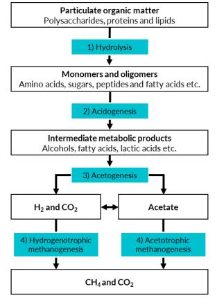
Figure 2. The biochemical process of anaerobic digestion
