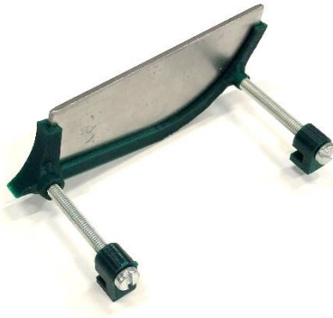
Figure 4.10. Parallel mounted metal plate.
