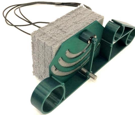
Figure 4.8. Reed relays and pendulum mounted in the duck.
