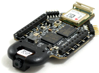
Figure 4.10: AI deck with GAP8 RISC-V MCU, ESP32 and an on-board camera. Image taken from [8], with Bitcraze's permission.
