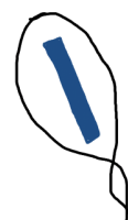
Figure 3.5: A schematic illustration of a crystal (blue rectangle) retrieved and positioned along the major axis in the loop.
