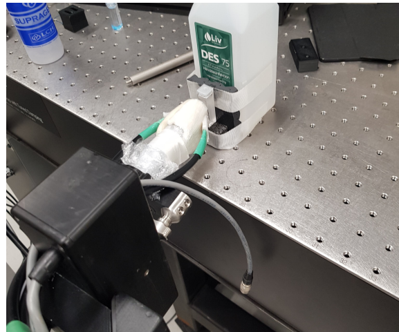
Figure 2: Picture of phantom and photoacoustic probe setup during measurements.
