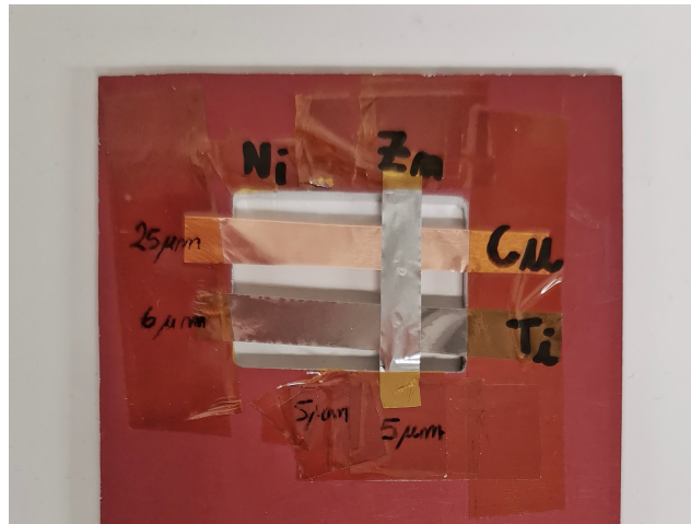
Figure 4.5: Ross filter used in the experiment. The Ross filter contains different metallic stripes. The copper stripe is 25\ \mu\text{m} thick, the titanium stripe is 6\ \mu\text{m} thick and the zinc stripe is 5\ \mu\text{m} thick. Originally, the filter included also a nickel strip, however it eventually got damaged so it was discarded. The stripes are held in place on the opening with kapton tape.
